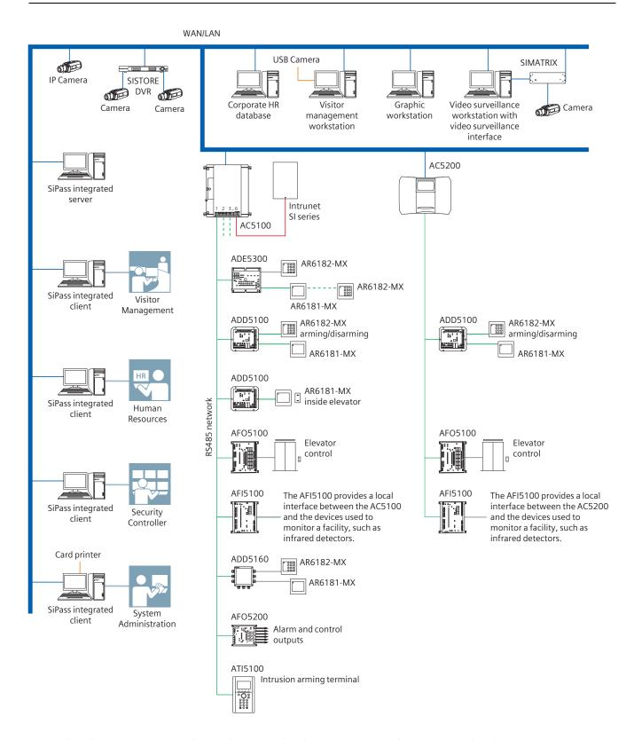
\* One of the six ports on the AC5100 is a multi-purpose IS interface that can be used for Intrunet SI series, high-level elevator control, Securitel or, if none of these are in use, for any other FLN.
