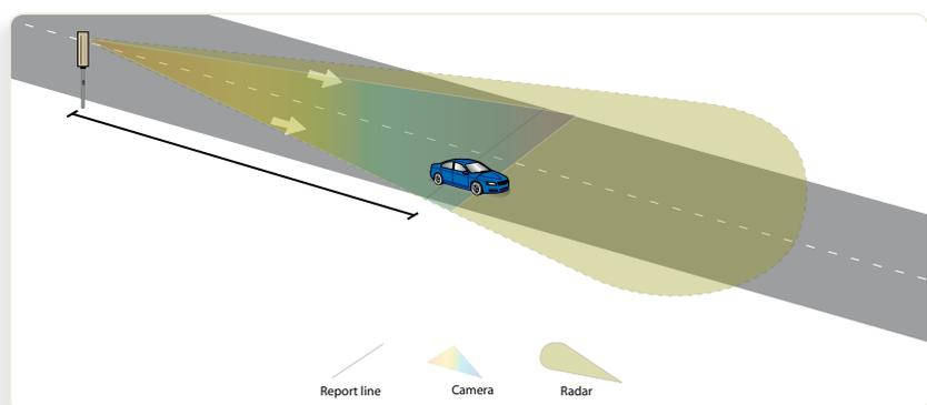
The SSS operates from the side of the road, tracking traffic for speed and distance.
