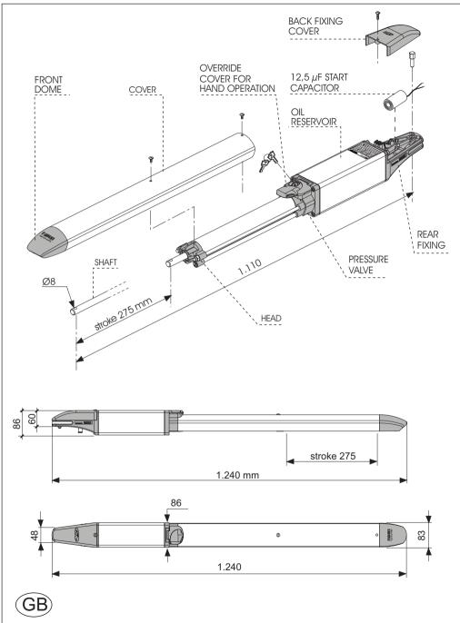
NUPI 66 is an oil-hydraulic actuator to automate swinging gates, designed and manufactured by FADINI with high precision technique. This product incorporates the motor, pump and valve assembly in one block, an innovative design, implying that all the parts work as a single unit immersed in an oil bath in the oil reservoir: oil is special and makes the unit unaffected by cold or hot weather.
