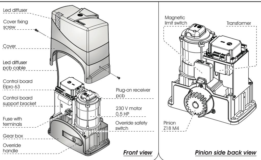
**JUNIOR 650** is an electro-mechanical geared motor to open and close industrial sliding gates having a max. weight of 1.200 kg. It is an electro-mechanical gate operator fitted with a 230 V - 50 Hz motor, designed and produced in full compliance with the EN12445, EN 12453 Safety Norms and the EN 13241-1 Product Norm: in case of an obstacle on opening, gate travel is reversed to allow the obstacle removal; on closing, travel is reversed and gate is driven to the fully open position.
