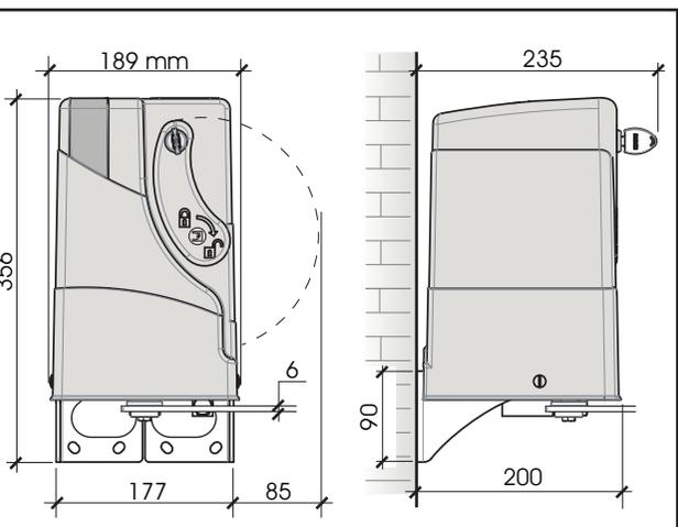
BART 350 is an electromechanical gate system fitted with an arm, either cranked or straight (both made of zinc-coated steel) for residential swinging gates, semi-intensive use, designed for gate post mounting.
