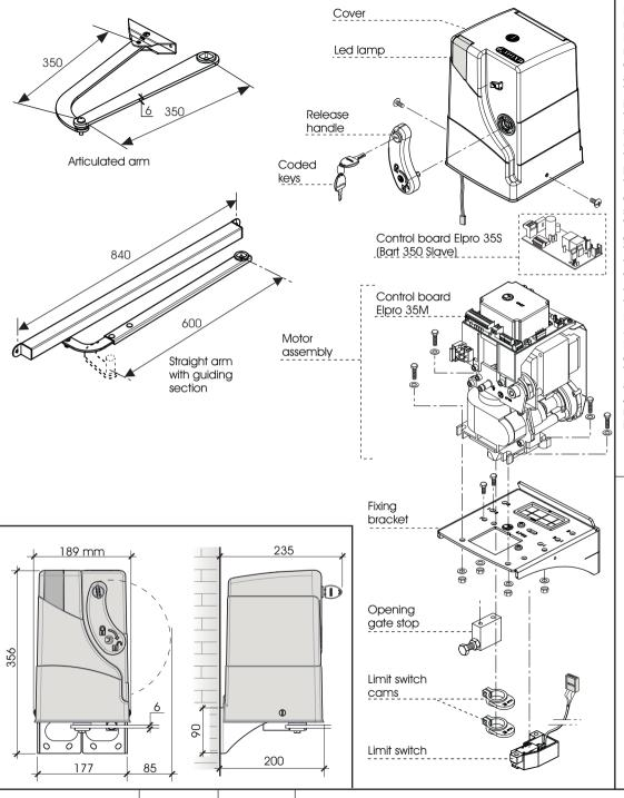
BART 350 is an electromechanical gate system fitted with an arm, either cranked or straight (both made of zinc-coated steel) for residential swinging gates, semi-intensive use, designed for gate post mounting.
